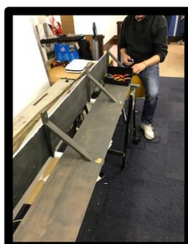
Back shelf for laptop. The gap will allow cables to pass through.
